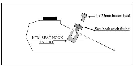
Hook slot on bottom of seat may need to be lengthened, allowing enough forward movement to install seat fastening screws. Connect fuel line from carburetor to petcock on IMS tank. Fill tank with fuel. Check for leaks. No leaks 1 Enjoy your longer ride.
