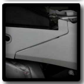
**Step 14**Align the tank shroud plastics in the back with the body shrouds so that there is as small a gap as possible. It may not be as
