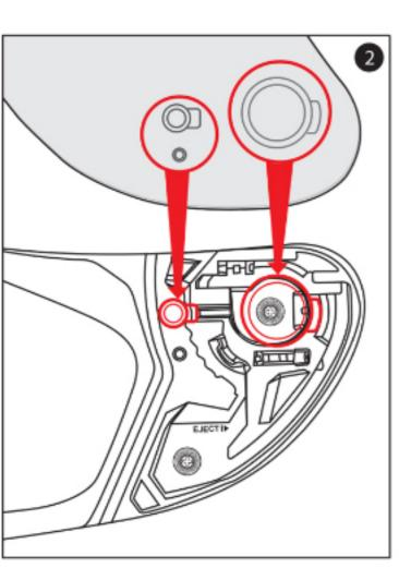
2. Align and insert the top of the shield guide into the plate-gear guide.
