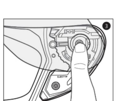
3. With the guides properly aligned, press the lower section of the shield into the plate-gear mechanism. The locking tab should pop into position, locking the shield into place.
