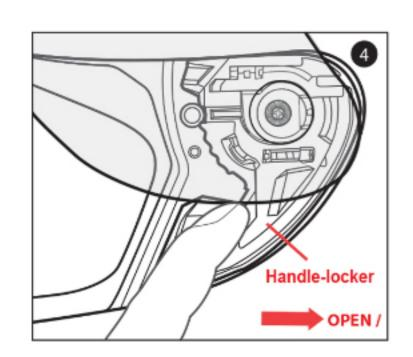
4. Push the handle-locker to the open position. The shield will be automatically released out of base ratchet mechanism.
