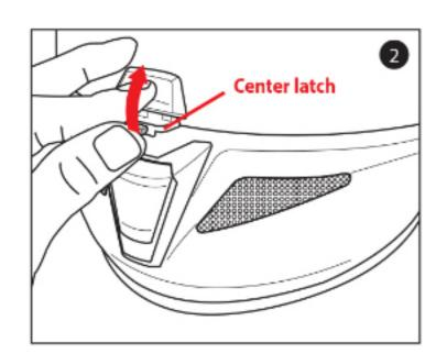
2. Squeeze the tab and lift up the center latch.
