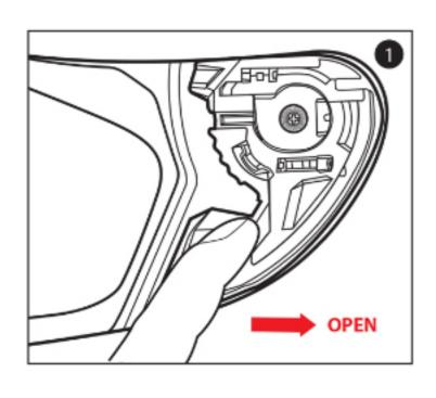
Ensure that the handle-locker is in the open position.
