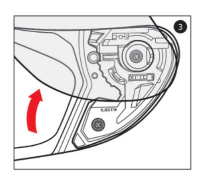
3. Open shield to the maximum open position.
