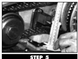
Place the other GUIDE PLATE with the bevel-cut edges facing inwards (towards the SHOE). Keeping the M6 held at a 90° (right angle) to the lower primary chain, torque the nut to 33 ft. pounds. Add a touch of loctite and you're done.
