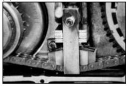
□ '85 and later rubber mounted engine option: If the lower chain when pressed down in the center clears the lower primary case by a minimum of 1/8", the SHOE can be installed upside down pressing the lower chain down. This would mean that the SHIMS would be on top with the springs underneath, then the SHOE. Use same spring compression measurements.
