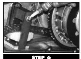
Oil and re-assemble the primary engine case. We recommend that you replace the gaskets. Check the unit for wear every 20,000 miles...and always keep clean oil. At some point in time you will have chain 'stretch' and will need to add an additional shim. Save your extra shims and instructions sheet for future use.
