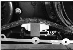
NOTE: The 3/8" is measured from the bottom of the shoe to the resting point of the springs on the guideplate, or shims (closest to the vertical bars).
