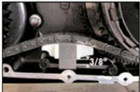
*NOTE: The 3/8" is measured from the bottom of the shoe to the resting point of the springs on the guideplate, or shims.*
