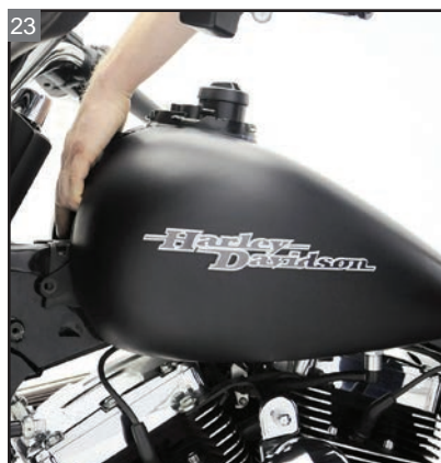
Remove the tank from the frame's backbone.
