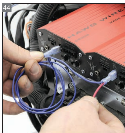
44 Plug the wires from the cigarette lighter into the REM (remote) port on the amp.
