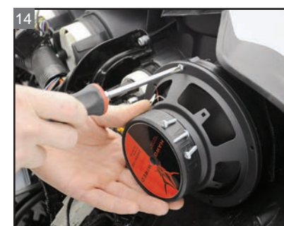
Install and tighten the Hawg Wired speaker.
