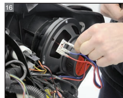
Plug the wiring from the crossover into the speaker.
