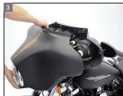
Remove the outer fairing and set it aside.
