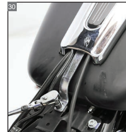
Install and tighten the dash's mounting hardware.
