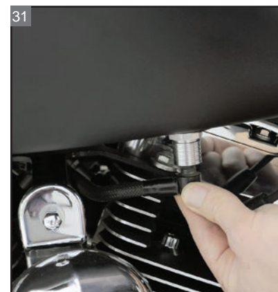
Plug the fuel line into the quick disconnect.
