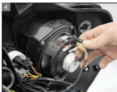
Unplug the speaker wiring.
