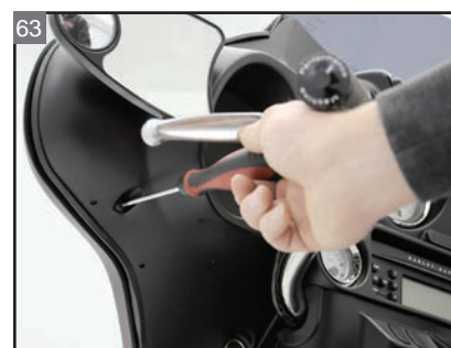
63 Install the outer fairing's mounting hardware.
