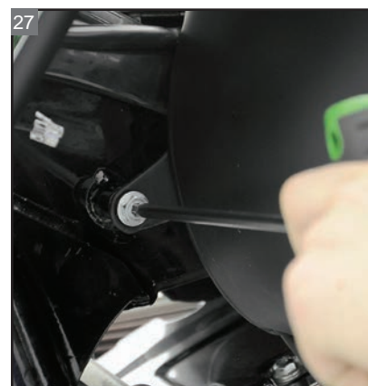
Install and tighten the tank's mounting hardware.
