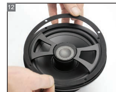
Install the foam gasket onto the speaker.
