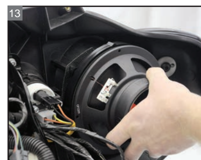
Position the speaker up to the adaptor ring.
