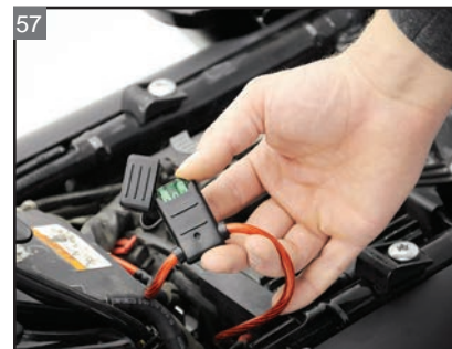
57 Install the fuses into the power wires.
