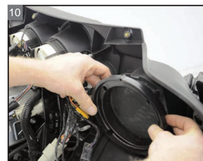
Position the adaptor ring so the longer portion faces upward.
