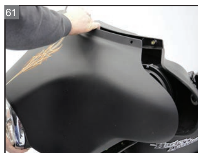
61 Install the outer fairing.
