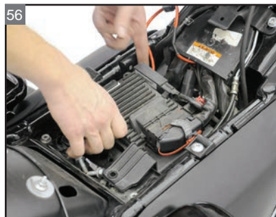
56 Install the ECM caddy and tighten the mounting bolts.
