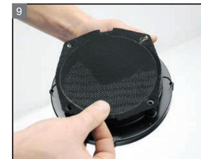
Place the speaker grill onto the adaptor ring.
