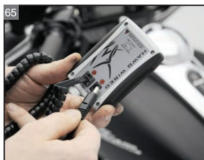
65 Plug the controller signal cable and power wire into the controller.
