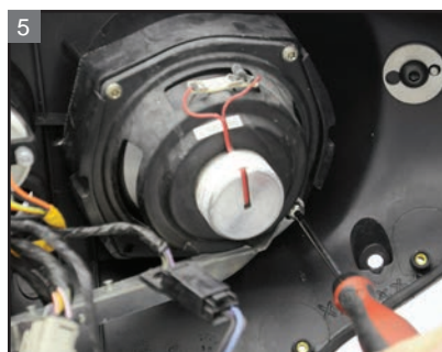
Remove the speaker mounting bolts.
