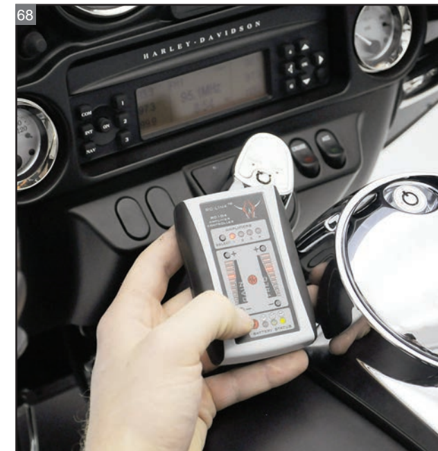
68 Adjust the amplifiers' gain and frequency.
