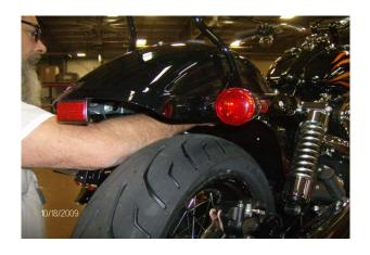
DETACH SHOCKS AND LOWER TIRE. REMOVE REFLECTOR AT REAR OF FENDER. REMOVE TURN SIGNALS REMOVE SIDE MOUNT LICENSE PLATE FRAME AND REMOVE LIGHT TO BE REUSED ON THE NEW FRAME.
