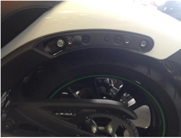
Fender Strut without cover. Note the larger hex head bolt to the front and the smaller to the rear
