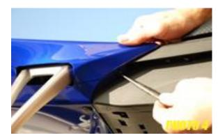
5. Remove the four 4mm allen bolts (photo 5). 2 on each side.
