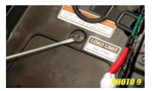
Unplug the wiring to the tail light assembly. Lift the tool tray and remove the 4 bolts with a 10mm socket. (photo 10). Hold onto the tail light assembly to keep it from falling after the bolts are removed.
