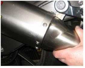
6) Torque first the mounting bolt and then the exhaust clamp to 20 Nm / 14 ft lbs. (photo 6)
