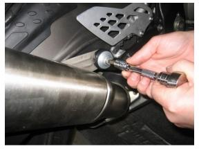
2) Loosen the exhaust clamp at the mufflers base and side muffler off. (photo 2)
