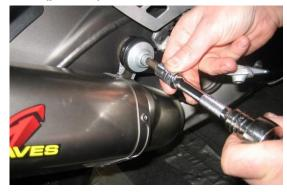
Make sure the slip-on has slid fully onto the stock exhaust system and it lines up with the heat shield.(photo 5)
