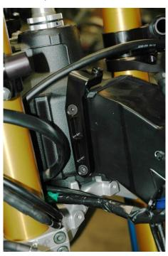
Install the fork clamp onto the left fork leg, under the handlebars. The fork clamp is mounted with the step pointing downward. 4) Install steering damper (see photo) and align the fork clamp. Apply thread locking compound and the pinch bolt torque (15 Nm / 11 ft lbs).
