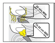
WARNING: Keep the bags a reasonable distance from the silencer. The heat and the exhaust could damage them.
