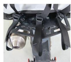
Strap on the Saddlebag, starting with the rear (see 3-Point Mounting), then connecting and tightening all connections until the Saddlebag is firmly attached to your bike. Tug the bag aggressively to verify that it's on there tight.
