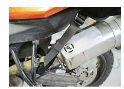
Loop lower left and right webbing straps Loop lower left and right webbing scape around or through the left passenger footrest bracket, NOT THE FOOTREST - the mount or bracket. Thread webbing through thumb-lock buckle — but do not full tighten yet.
