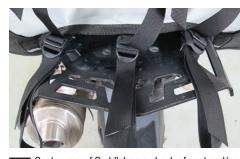
Center rear of Saddlebag on back of seat and/or Center rear of Saddlebag with at least tail rack. Connect rear of Saddlebag with at least 1 strap affixed to center of rear rack, passenger grab handles or other secure anchors. If possible, use all 3 straps on the rear of the Saddlebag. Although the side straps do most of the work "hugging" the bag to the bike, the rear strap(s) stabilize the load and prevent the Saddlebag from shifting forward while riding.
