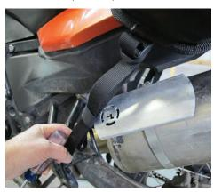
Note where the Saddlebag and/or straps may potentially make direct contact with exhaust components. Install one or more Hot Springs Heat Shields to protect any/all parts of Saddlebag from touching any/all parts of the exhaust system (see below).
