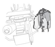
5 CONNECT TOP STRAPS Connect top compression straps over top of luggage rack
