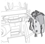
NOTE: If any part of the Pannier or strap touches exhaust, install a Giant Loop Hot Springs Heat Shield to prevent damage. (optional accessory, not included with Panniers) to prevent damage.
