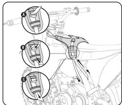
Locate the appropriate connection points on each side of frame. Use the farthest forward positions available (i.e., the shortest distance). Loop each side's webbing straps around frame/subframe and back up through reflective tabs and thumb-lock buckles. DO NOT allow webbing to contact exhaust! Tighten all three points of contact and secure all loose webbing ends.
