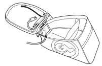
Pass power cable into mesh pocket on underside of Tank Bag lid by thread through either side of yellow sleeve.
