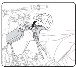
3 The Kiger/Fandango/Diablo Tank Bag is designed to allow easy access to your fuel filler by simply unzipping one side of the bag from the harness. Note that the concave shape of the Tank Bag's front allows vent tubes to breath. Unzip the Tank Bag on both sides to remove it from the harness and take it with you, leaving the harness mounted and ready to go.
