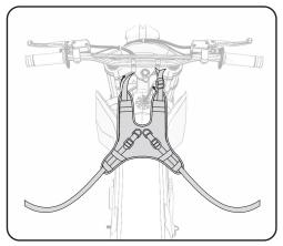
1 Thread the forward webbing under the frame head tube and back into the thumb-lock buckle on harness. Adjust the front mount point to fix the front/back position of the harness to provide fuel fill access and full swing of the handlebars. Do not damage or interfere with any wiring, cables, other controls.
