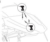
Using the included hardware, secure the Tail Rack with the round headed bolts on top, the spacer between the Tail Rack and fender, and washer and nut on the underside. We recommend using thread lock to prevent vibrations from loosening bolts on the trail.
