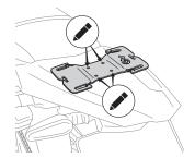
Remove the Tail Rack and drill holes through the fender. Double check positions under fender before drilling to ensure wiring or other components will not be damaged.
