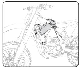
Secure front Pocket straps around cowling, tank vents, tank or radiator mounts. Tighten straps and secure loose webbing ends. Reinforce and stabilize with Pronghorn Straps, if needed.
