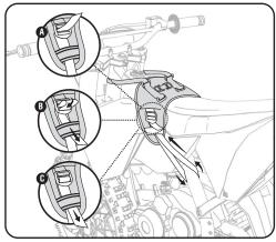
2 Locate the appropriate connection points on each side of frame. Use the farthest forward positions available. Loop each side's webbing straps around frame/subframe and back up through reflective tabs and thumb-lock buckles. DO NOT allow webbing to contact exhaust! Tighten all three points of contact and secure all loose webbing ends.
