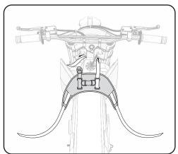
Thread the forward webbing around the frame head tube and back into the thumb-lock buckle on harness. Adjust the front mount point to fix the front/back position of the harness to provide fuel fill access and full swing of the handlebars. Do not damage or interfere with any wiring, cables, other controls.
