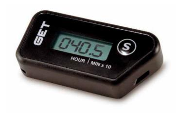
C1 is the famous wireless engine hour meter by GET. C1 can be easily installed and captures the frame's vibrations, distinguishing typical engine vibration from other random ones. The device is waterproof and is conceived to work in the harshest conditions. C1 has two hour meters, one measuring global working time and the other one resettable.
