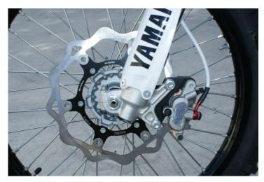
Be sure to pump the brake lever a few times, making sure the system is working properly. Please be aware that the overall braking feel has been changed dramatically. We suggest taking it easy while you get used to the new brake lever pressure and feel.
