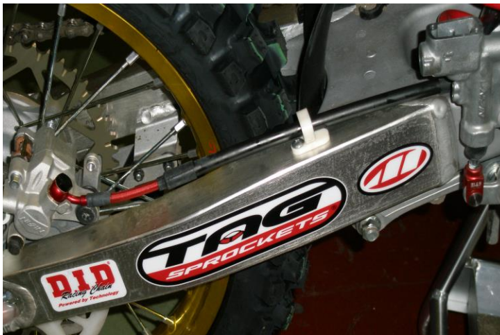
C. Line routed down the swing arm to caliper
