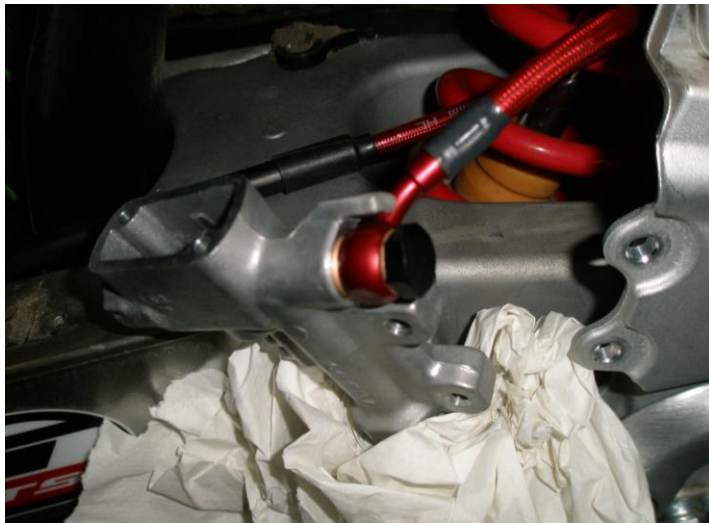
A. Rear Master Cylinder (removed from frame)
