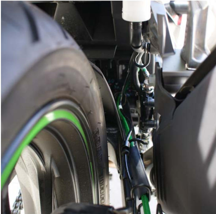
I. Line D routing down the Swing Arm
