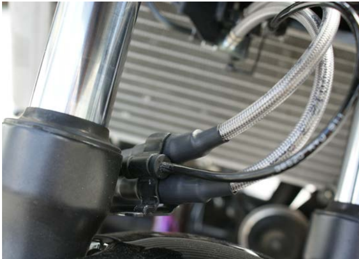
i. Lines B & C routed through OEM bracket at front fork
