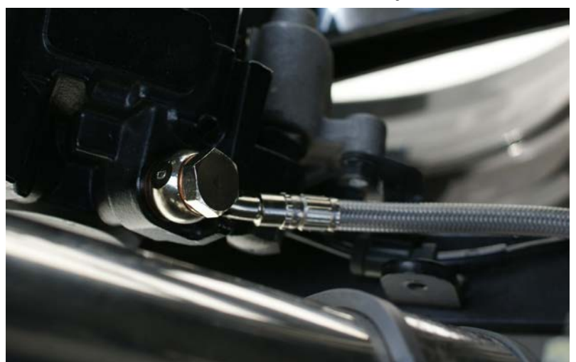
n. Line E installed at rear caliper
