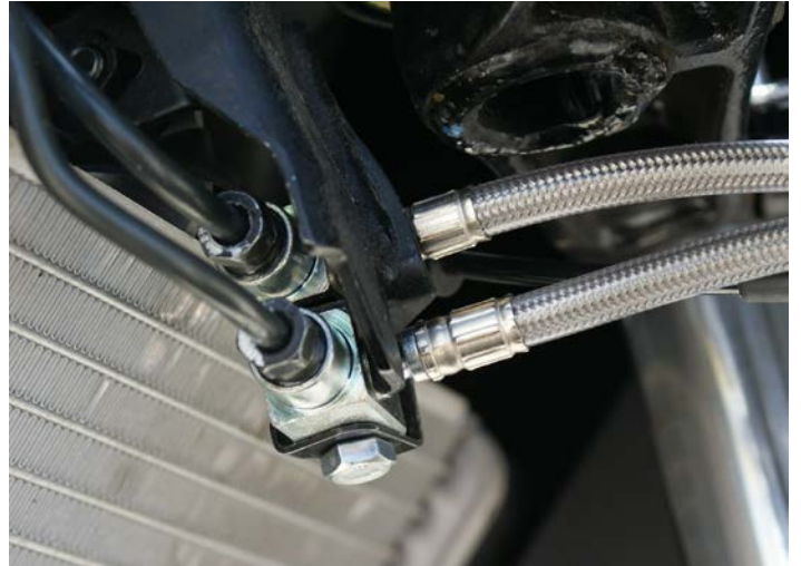
j. Galfer M16 bolt installed to OEM bracket at the lower triple tree
