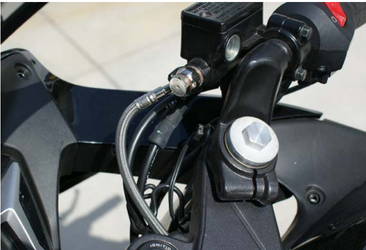
a. Line A installed to front master cylinder
