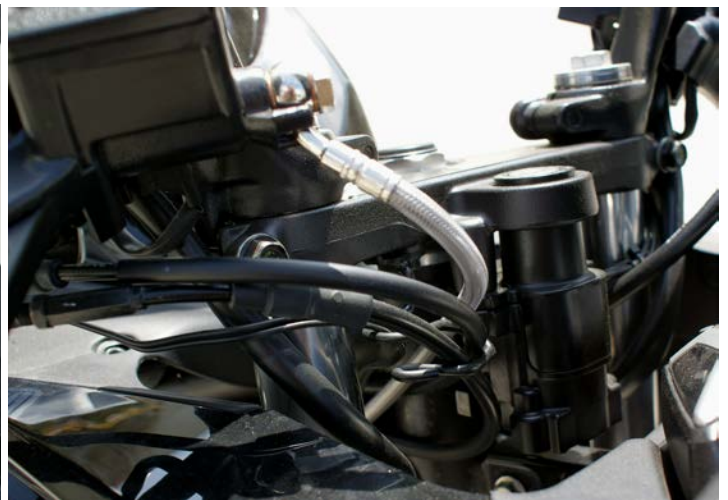
b. Front master cylinder routing
