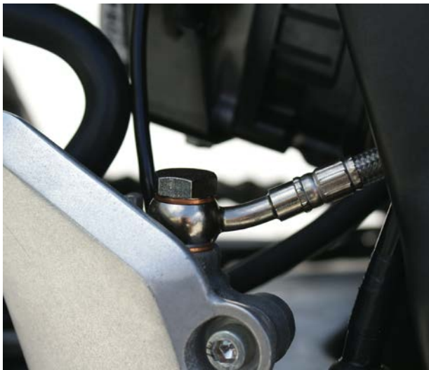
k. Line D installed to rear master cylinder
