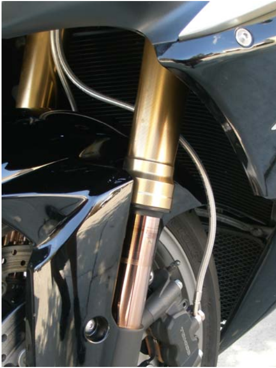
e. Left caliper routing
