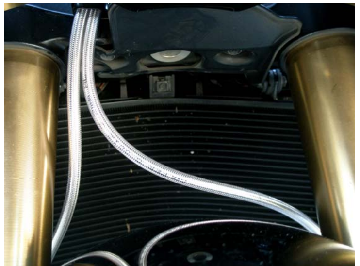
d. Galfer lines routed behind the forks
