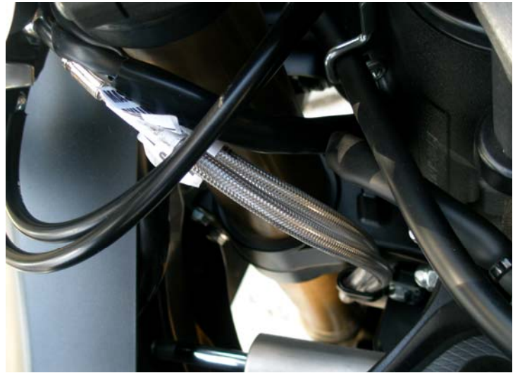
b. Routing from master cylinder to lower triple tree
