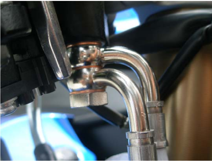
a. Front master cylinder, notice positioning and sequence
