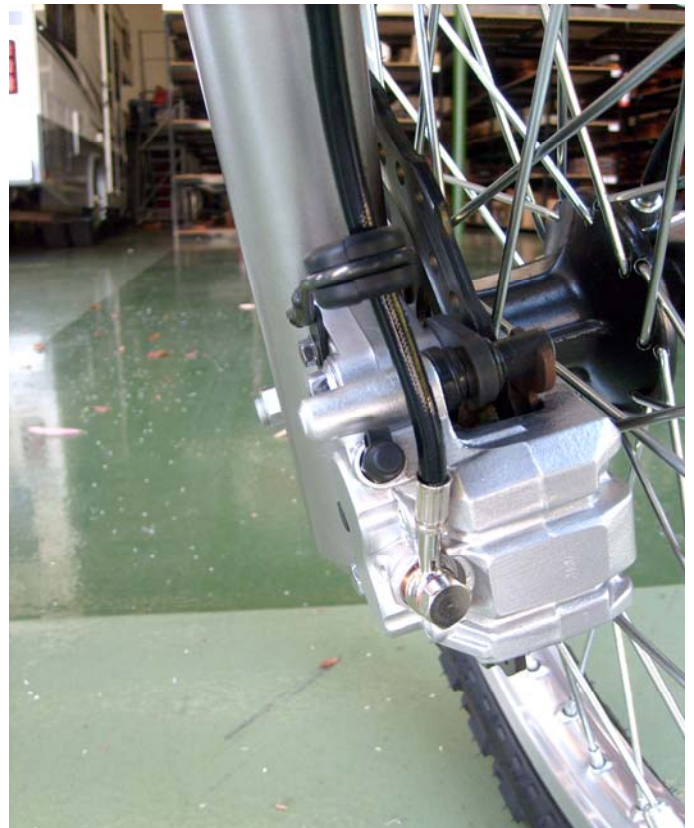
d. Left caliper, line routed through OEM line holder
