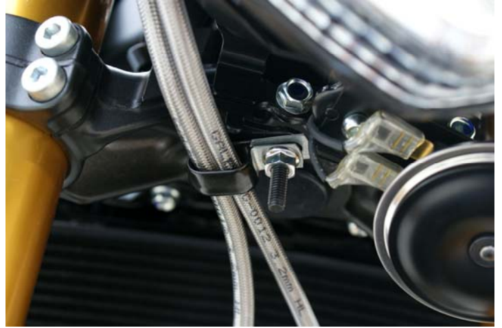
b. Galfer c-clip at lower triple tree
