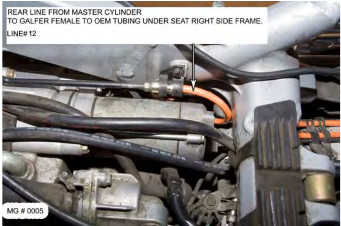
(Fig: MG0005) Line# 12 rear line from master connected to OEM tubing with brass olive right side frame under the seat.
