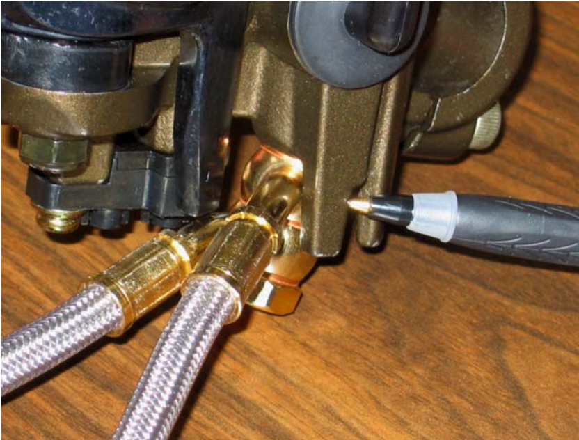
Master Cylinder Modification Picture to the right: Galfer lines installed with master cylinder on bike, pen and “X” indicate which tab to grind off, notice sequence and position of fittings
