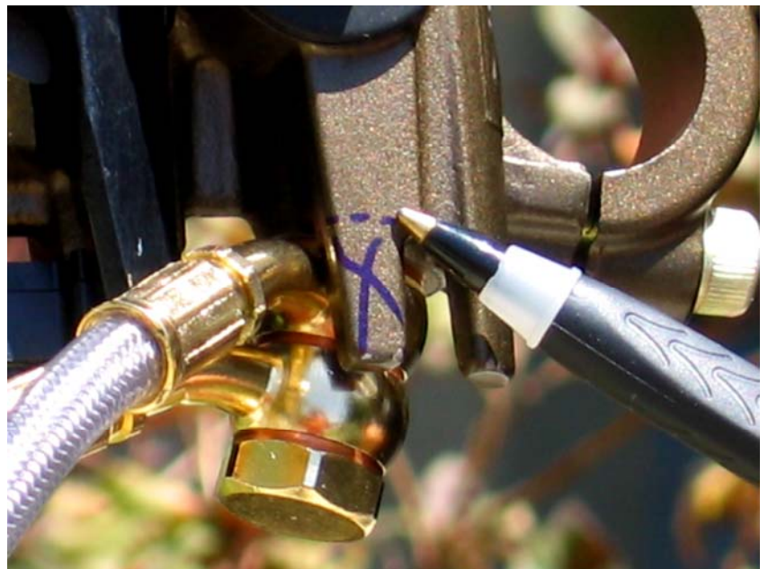
Master Cylinder Modification Picture to the right: Galfer lines installed with master cylinder on bike, pen and “X” indicate which tab to grind off, notice sequence and position of fittings
