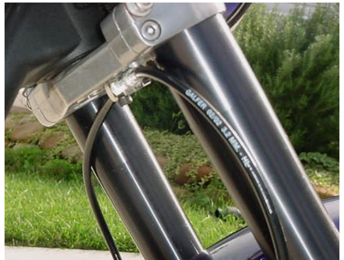
d. Lower lines routed behind the forks
