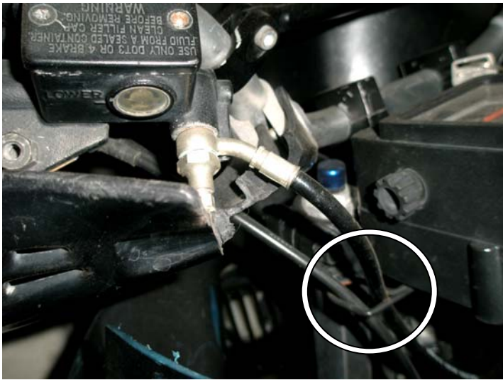
A-1. Front master cylinder (with Galfer bleeder,) Galfer line routed at control panel with throttle cables in circle
