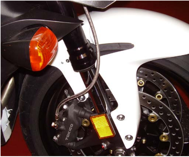
D. Line Routed in Front of the Fork to the Right Caliper
