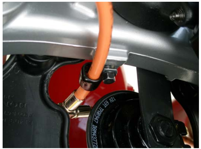
b. Top line routed through the Galfer c-clip at lower triple tree
