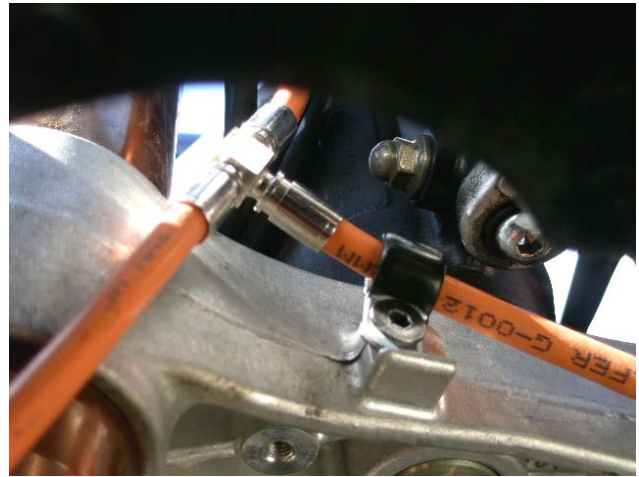
b. Galfer c-clip at lower triple tree
