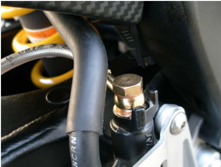
A. Rear master cylinder, notice position of fitting
