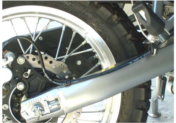
b. Galfer line routed down swing arm, notice OEM clip by the master and the Galfer provided c-clip by the caliper
