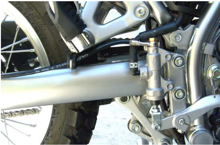
a. Rear master cylinder, Galfer line routed through OEM routing clip
