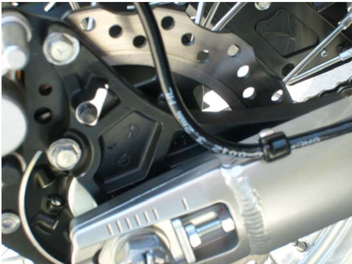
c. Galfer provided c-clip at the swing arm, notice OEM bracket at the caliper assembly has been removed
