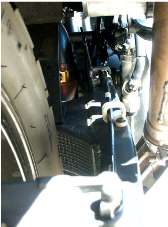
c. Rear routing, using OEM routing clip
