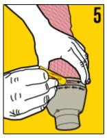
Before reinstalling the inner core assembly into the muffler can, apply a thin bead of FMF high-temp silicone on the front end-cap where it makes contact with the canister.
