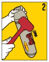
Using care not to damage or distort the shape of the metal, grasp the front end-cap (midpipe side) with your hand and begin working it out of the muffler canister. You may need to lightly tap the muffler mount with a rubber mallet for an easier separation. Slowly pull the end-cap and core all the way out of the can, exposing the remains of the old packing material.
