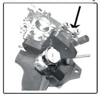
If the valve leaks use a punch to re-seat the valve
