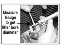
Measure lifter O.D. & Subtract from Bore size to get clearance
