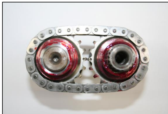
'07-'16 + conversion camshafts, inner cam chain #8060 installed with camshaft timing marks aligned. Lead with rear cam when installing into camplate
