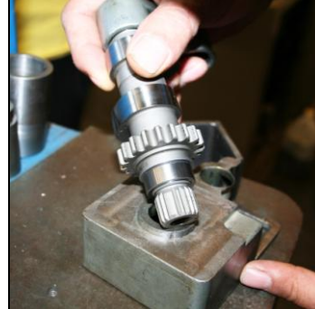
Set camplate into proper fixture to press roller bearing into camplate, verify bearing is pressed square and flush with camplate
