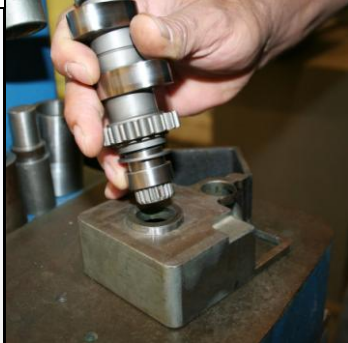
Set camplate into proper fixture to press roller bearing into camplate, verify bearing is pressed square and flush with camplate
