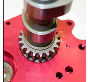
Set camplate into proper fixture to press roller bearing into camplate, verify bearing is pressed square and flush with camplate
