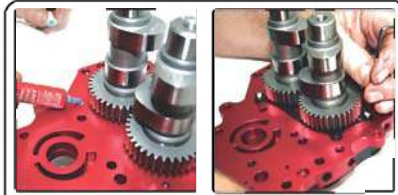
Install bearing retainer plate using loctite
