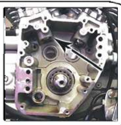
Verify Intake lobes of camshafts clear engine case Crank bearing boss & lifter bosses
