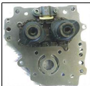
Install inner hydraulic tensioner unit
