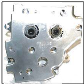
Install cam bearings, camshafts and front cam outer retaining ring
