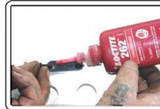
Apply Loctite to block off plate bolts
