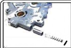
Inspect pressure relief valve
