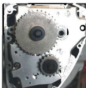
Align the outer chain sprockets using the proper thickness sprocket alignment spacer
