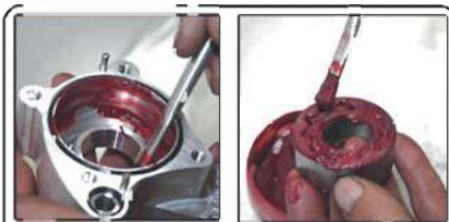
Apply engine assembly lube to oil pump housings & gears
