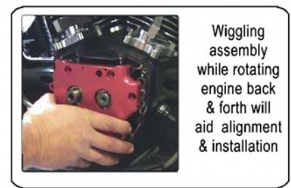
Install camplate & oil pump as a complete assembly
