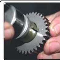
Line up gear with camshaft
