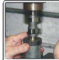
Press cam gears onto camshafts
