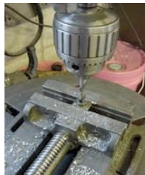
FIGURE 2-drill rear fender nuts
