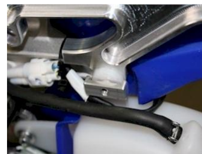
FIGURE 3-Coolant tank nut installation
