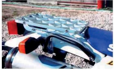
spacer on the bolt and then screw the bolt into the hole on the frame of the bike. Leave them loose for now. Do this on both the left and right side of the bike.
