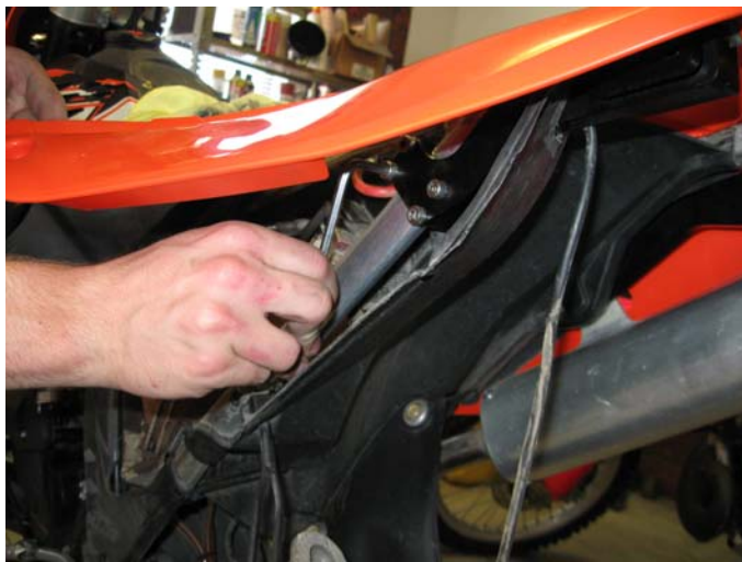
FIGURE 8: LH sub frame bracket clamp
