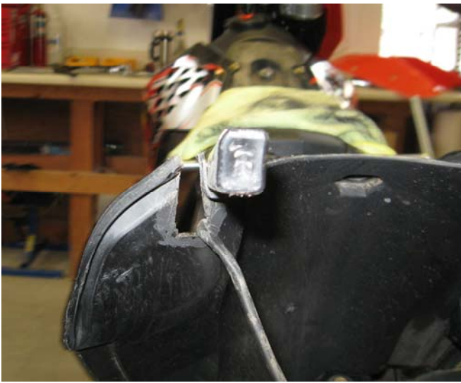
FIGURE 2: LH air box cut-out
