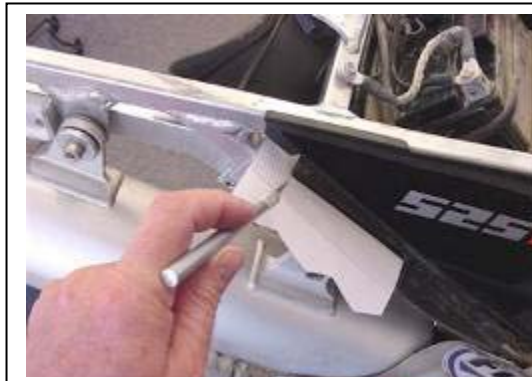
Figure 8: RH air box trim template taped to plastic
