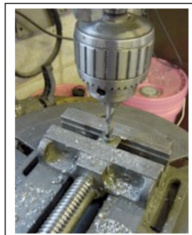
FIGURE 2 Drill rear fender nuts
