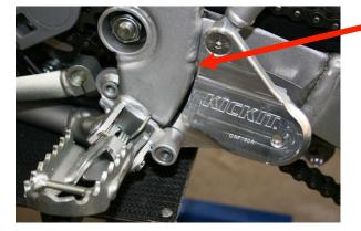
**VERIFY:** Weld does not interfere.
