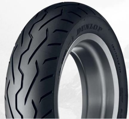
A radial tire that delivers performance and provides handling, riding comfort, and speed capability.
