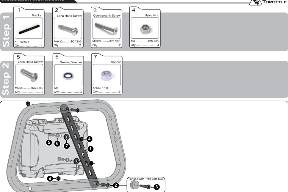
**Step One:** Bolt the mounting bracket to the rack using the included hardware. See diagram for installing with Trax Side cases. **Step Two:** Place the case against the bracket and mark the hole pattern on the case. Using a 6mm drill bit, drill through the back side of the case. Using the included hardware, bolt the case to the rack.
